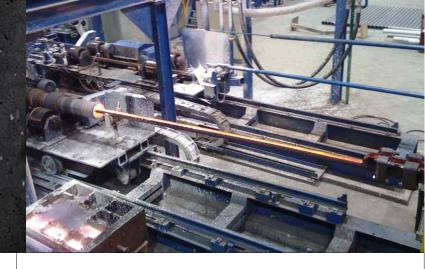
TROUGH BLACKINGS are a fully prepared Coating based on blend of Carbon and refractories for use on metal or ceramic lined Troughs and Fall Chutes during the production of Centrifugal cast pipes using Delavaud process.
