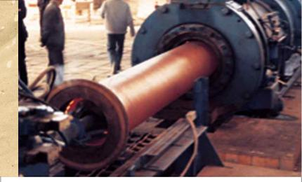
**DIECOTE** is a range of Hydro based coating for permanent metal mould during Centrifugal Casting applications.
